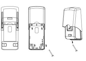
Step2: Install the waterproof cover replace the plate on the T50 device and fix back plate with 4 screws so that the waterproof can be slide up and down and fixed the T50 front plate on the back plate board.
