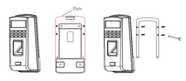
Step1: There is a plate at the back of the T50 device. Please remover it before install the waterproof cover.
