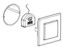
Fig.3 Installation of Fibaro Roller Shutter in wall switch box.
