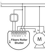
Fig. 1 Roller Shutter wiring diagram
