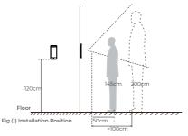
Suggested installation height (the distance between the lens and the ground) is 1.4m, as the recognizable body height range, 0.5m distance away from the device, is 1.3m-1.7m; the recognizable body height range, 1m distance away from the device, is 1m-2m. (There are some deviations)
