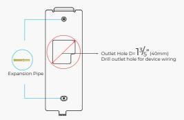
Please punch out the tail lines from the outlet hole before installing the mounting bracket and use the screws to fix the mounting bracket on the wall. Use the screwdriver to tighten thescrew follow the direction indicated, to complete the installation.
